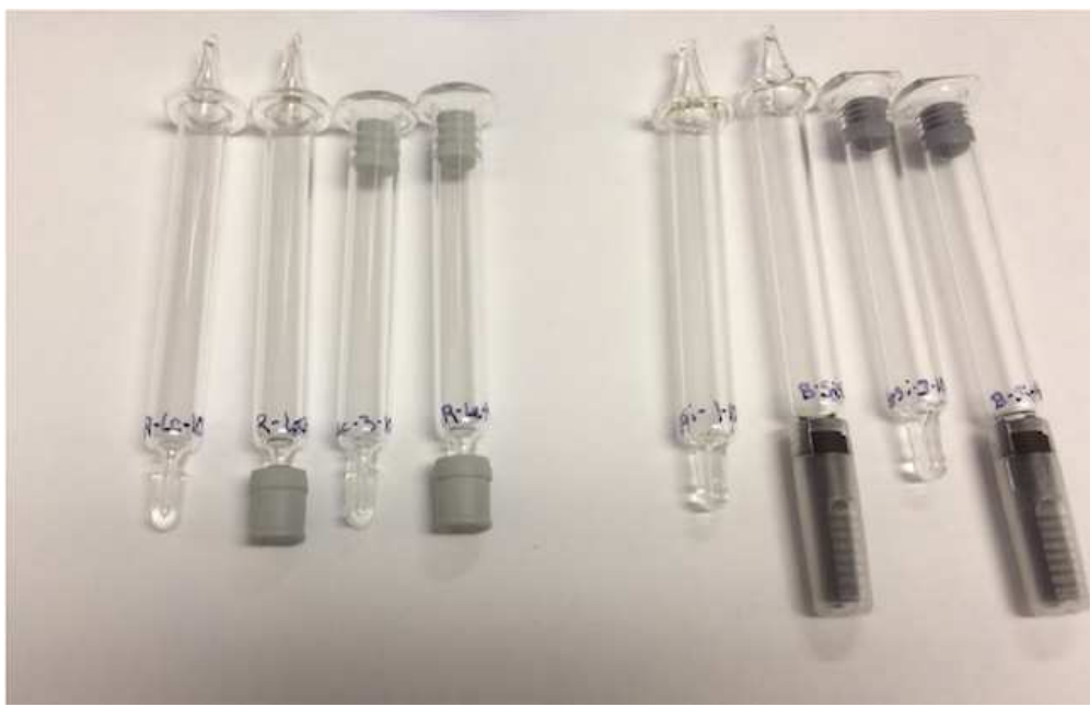
Negative controls were flame sealed on both ends. Positive controls were flame sealed on both ends and had 2, 5 or 10 micron laser drilled holes in the syringe body (Lennox Laser). All syringes were flushed with nitrogen before flame sealing. Oxygen ingress was measured over time.
